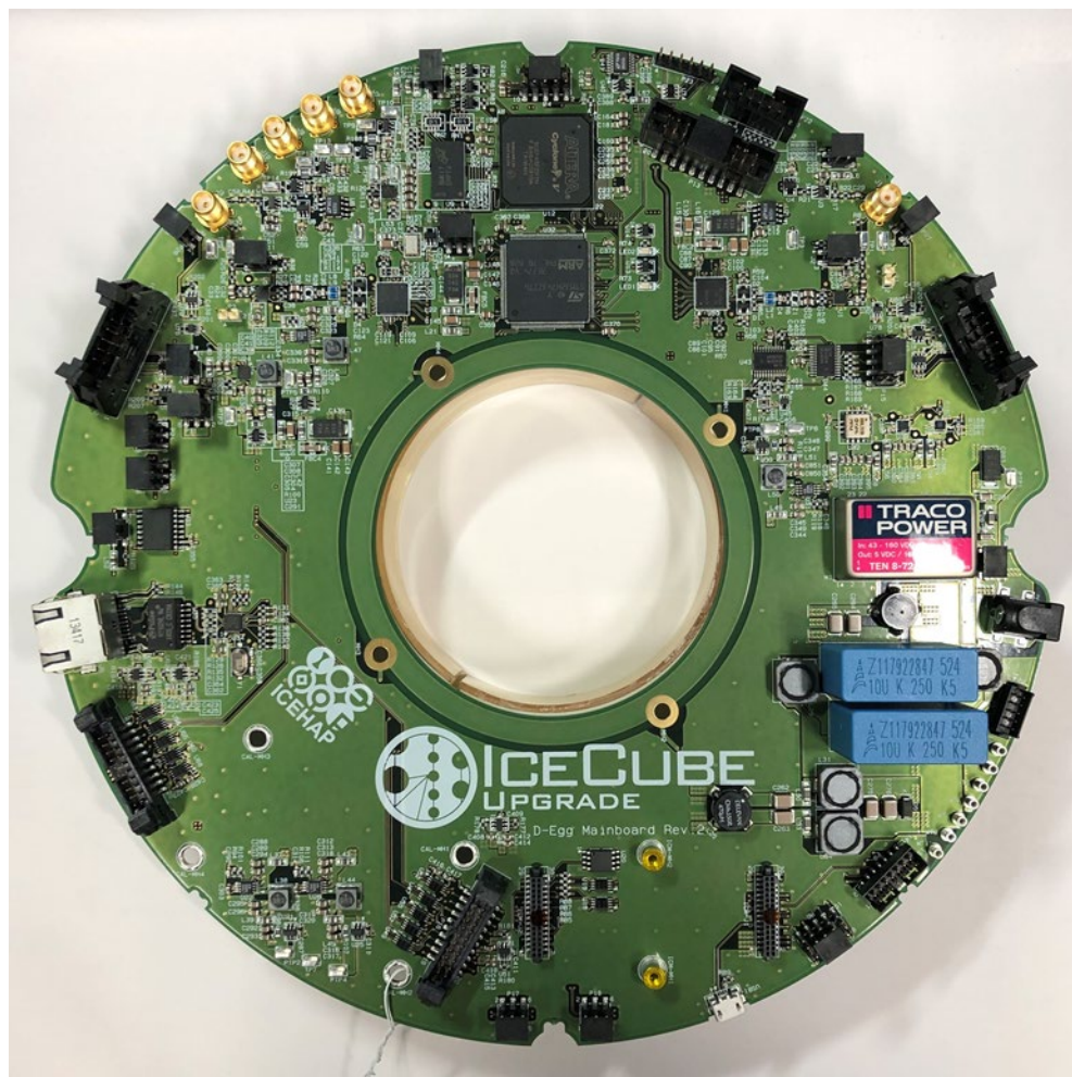
Figure 7: The second revision of the D-Egg in-ice optical module main electronics board, produced at the University of Chiba, currently undergoing testing.
