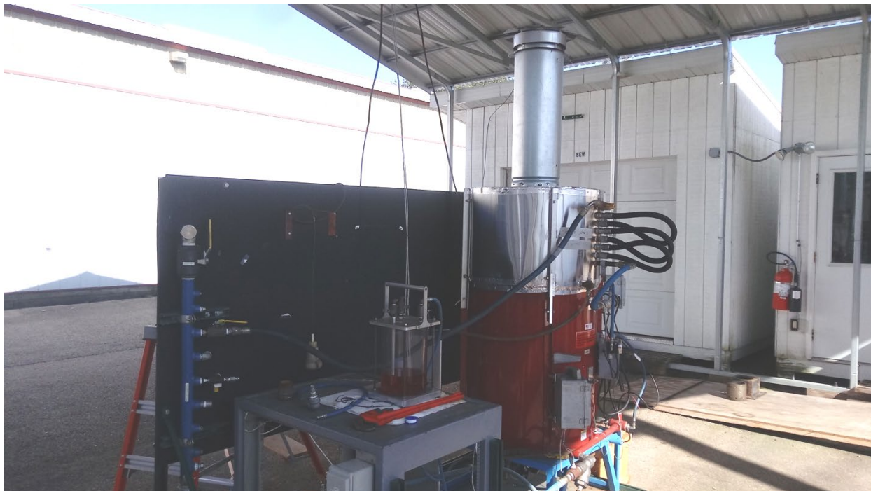
Figure 4: Heater assembly under testing at the IceCube test bed at UW's PSL. A complete slice of the enhanced hot water drill is kept operational in Madison for training and upgrading purposes.
