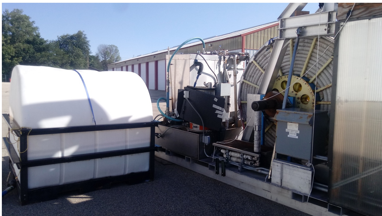
Figure 3: The IceCube Upgrade firm drill undergoing test operations at University of Wisconsin-Madison's Physical Sciences Laboratory (PSL). This subsystem will ship this fall for Antarctica.
