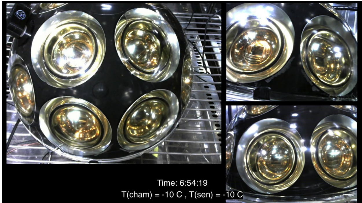
Figure 6: In-ice optical module mDOM test article undergoing cold tests of new optical gel materials at the University of Muenster.
